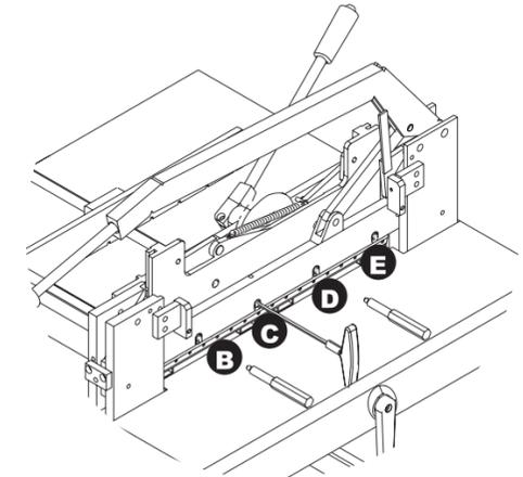
(16) Return the knife lever to its starting position and lock it.
