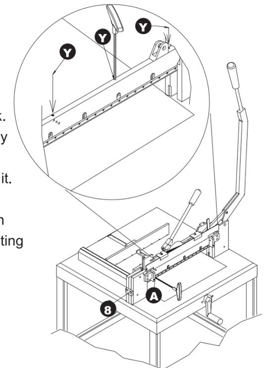
(22) Assemble Hand Guard and Cover by way of screwing in screws **a** **b**.
